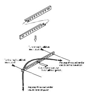
Figure 4. Rear Cable Support Bar.
